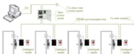
**Figure 6: Access control system using serial main controller and intelligent readers**
