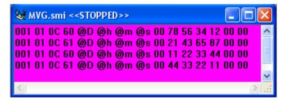
A line contains an event of a card being entered: Mux number 001, controller number 01 (to which reader is connected), length of message (0C hex is 12 bytes), message type (60 is reader 1 requested, 61 is reader 2 requested), @D inserts the PC date, @h the hour, @m the minute, @s the second, 00 reference not used, card number (of 8 digits in BCD), 2 bytes not used.
