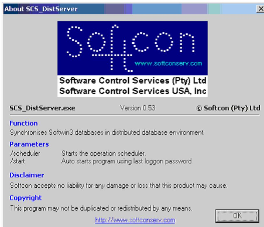
**Help about** displays the software version, the basic functions of SCS\_DistServer and the parameters that can be passed when the program is run. Parameters are separated with spaces.
